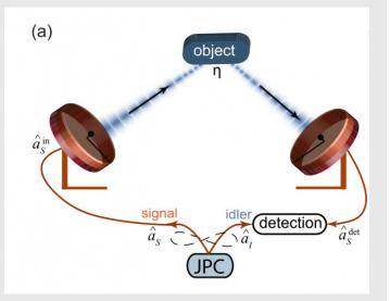
This "quantum entangled pair" interacts in a process called quantum illumination, where information about one particle's environment can be inferred by studying the other particle.
