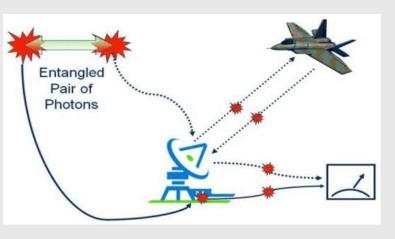
of de-coherence. This is the loss of "quantumness," or coherent entanglement of the photon pairs, as the transmitted photon passes through a lossy medium, such as the atmosphere.<sup>[iii</sup>]
